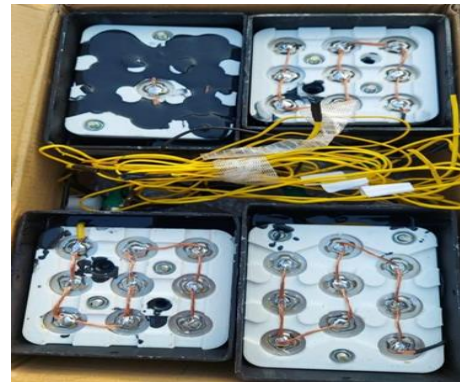
Fig. 1 Experimental setup for temperature measurement in Li-ion battery
